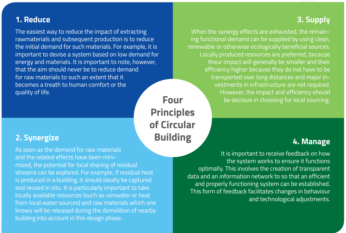
Figure 3. The principles of circular building as seen in Gemeente Amsterdam (2017). Roadmap Circular Land Tendering – An introduction to circular building projects (12) .
